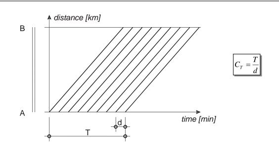
Actually, this simple formula may be misleading. When intermediate stations have a single platform for train stops, overall capacity of the line may be set by the station capacity: following trains cannot enter the station until the previous one leaves. Stop duration, and therefore passengers' exchange, may be a critical factor in determining minimum headway.
