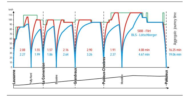
Figure 5 Comparison of speed-space diagrams for Flirt and Lötschberg EMUs
