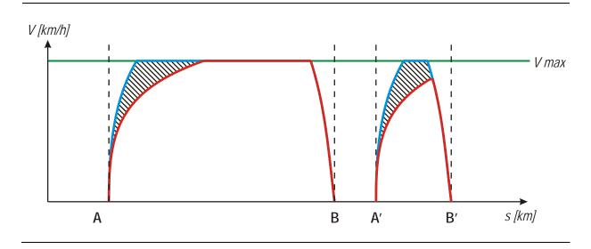
Figure 4 Speed-space diagrams for various acceleration rates
